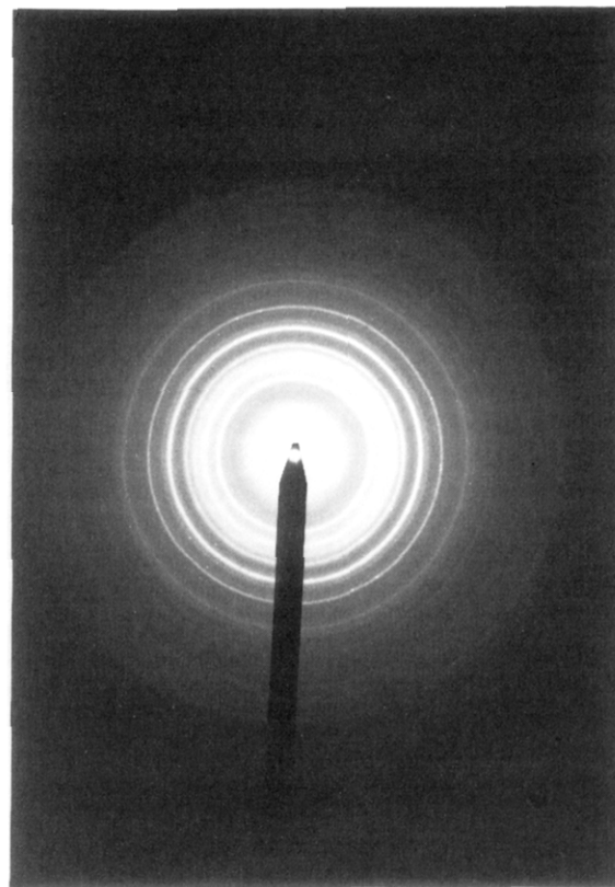
Figure 10. Electron diffraction patterns of the film grown from [(t\text{-Bu})\text{GaS}]_7 at 390 °C after thermal annealing (30 min at 475 °C).
