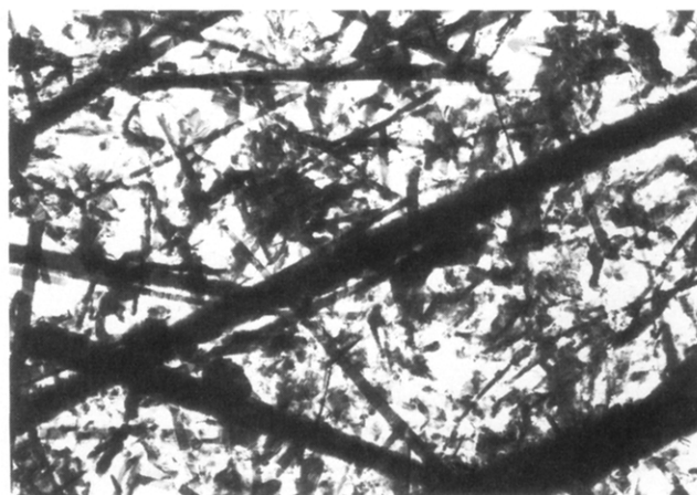
Figure 8. Bright-field TEM image of the down flow growth region of films grown from [(^t\text{Bu})\text{GaS}]_4 at 500^\circ\text{C} .
